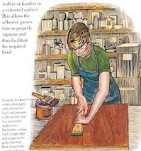
cement because it is readily available and is the easiest to use. Ir this application, contact cement, a flexible adhesive, will be used to bond a flexible overlay to a rigid substrate.
